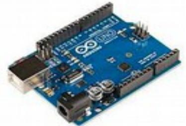
You will also notice the rows of header pins on each side, with this standardized format a large variety of daughter boards, called "Shields" can be plugged directly onto the main board. These shields can offer functions like WIFI, ethernet, motor shields, servo shields, and others that can greatly expand the available functions.
