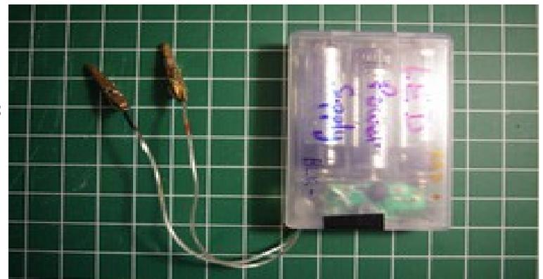
Normally I file the plastic drop flat above the LED to provide a better surface to glue the LED to whatever I happen to be working on. I then cut the leads flush with the plastic drop on one side and short on the other, scrape off the insulation using a knife blade and then solder on very flexible wire to the leads. Make sure to determine the LED polarity using a battery tester so you can get your wire color correct. For locomotive use, I
