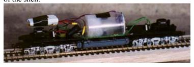
The sound decoder is a Soundtraxx DSX unit (just a sound decoder, no motor controls), with sound for 1st Generation EMD Diesels. It is mounted on a piece of metal, which I formed into a "Z" shape and attached to the frame. I ordered new E9A powered trucks from Life
